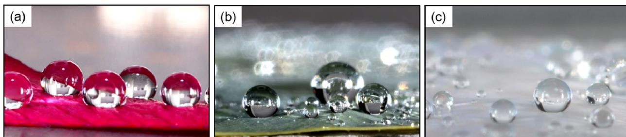
**Figure 9.** Digital photographs of typical water droplets on (a) a rose petal, (b) a lotus leaf, and (c) a PS film roll-pressed at  $T_p=180$  °C.
